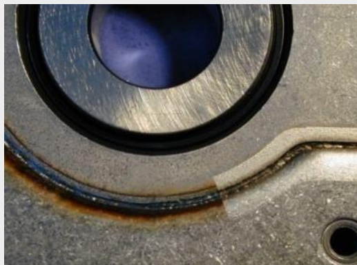
Soldering Seam Cleaning
