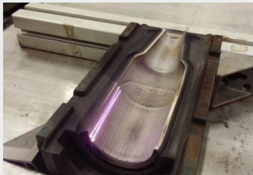
Mould Degrease Cleaning
